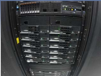
Lenovo Flex System: 12 Blade servers each 28 cores @2.6GHz, 128GB/1TB memory
