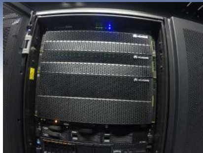
OceanStor 2200 Storage: 30TB redundant
